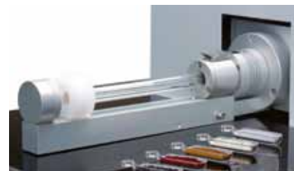
Double furnace technology – sample feeding for determining TOC in solids
