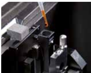
Adjustable cell holder with ultra-micro cell for extremely small sample volumes
